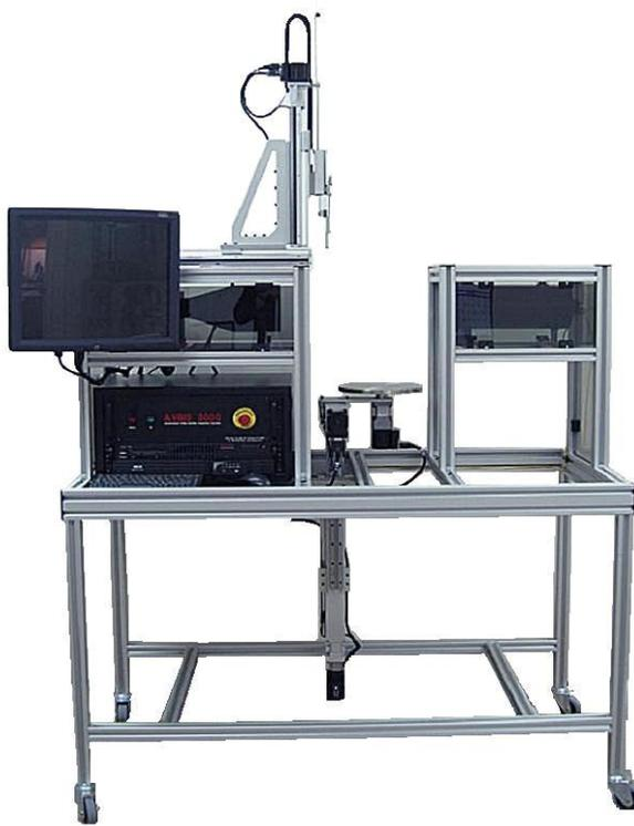
The AVBIS 3000 M is AVID Corporation's basic automated vision bottle / preform measurement system. Designed to measure neck finish and body dimensions accurately, repeatably and quickly, the AVBIS 3000 M is an ideal choice for quality attentive packaging manufacturers looking to improve their measurement capabilities. The small footprint and low-cost (<\$65K for the base system) of the AVBIS 3000 M suits those laboratories with space and budget constraints.
